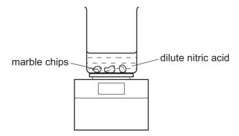
50 cm³ of dilute nitric acid, an excess, was poured into a beaker. The beaker was placed on a balance and the marble chips added to the beaker. The apparatus was weighed immediately and a timer started. The mass of the beaker and contents was measured every minute for ten minutes.
